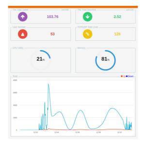
With around 50 simultaneous connections, the PoE extender had around 20% CPU utilization and 80% memory utilization. This is a good balance to ensure efficiency.
